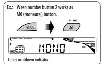
To use these buttons for their original functions again after pressing MODE, wait for 5 seconds without pressing any of these buttons until the functions mode is cleared or press MODE again.
